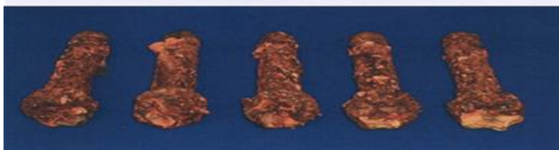
Figure 14: SL std (Z + 5000 hrs per ASTM B117)
