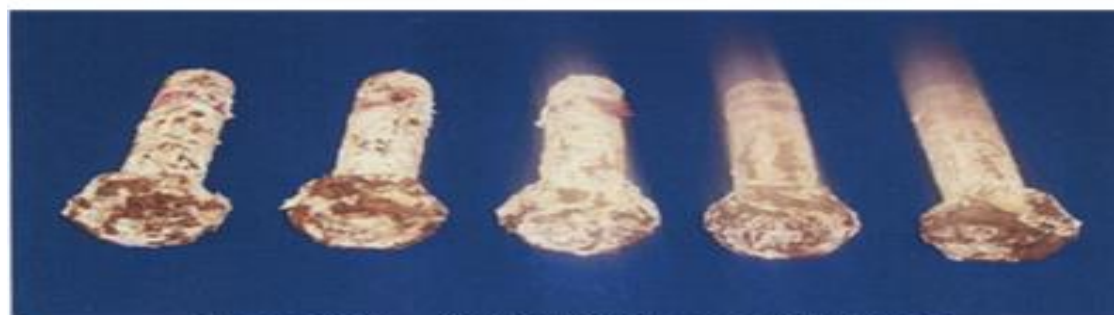
Figure 13: SL std (HDG + 5000 hrs per ASTM B117)
