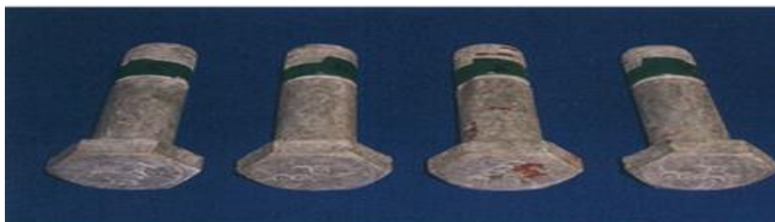
Figure 12: SL std (DACROMET® + 5000 hrs per ASTM B117)
